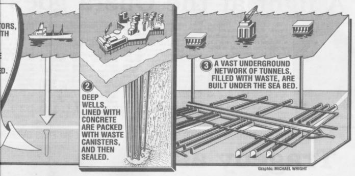
THREE different schemes are being considered by engineers for dumping nuclear waste in the seabed.
